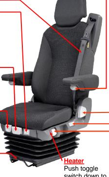
Push toggle switch down to turn on and the up to turn off.
